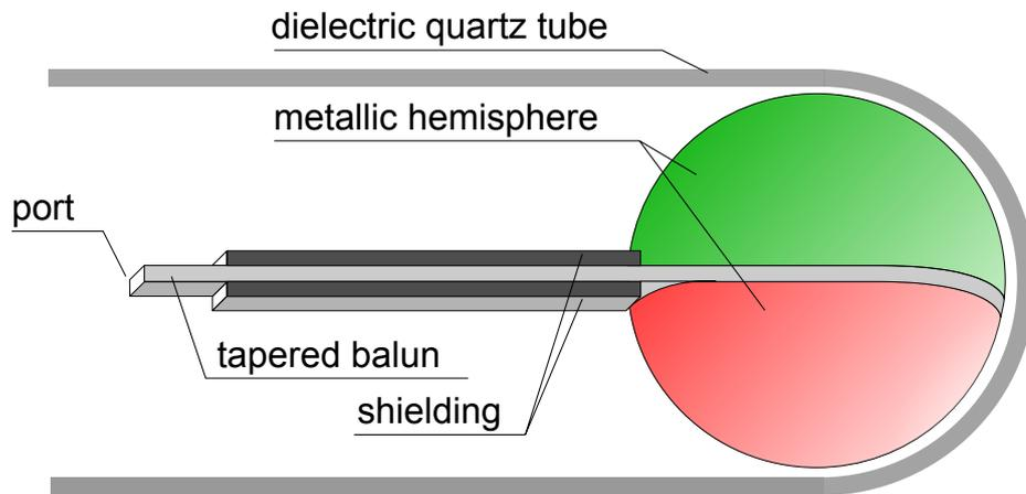
*Figure 1.3:* Prototype of the MRP: The probe consists of two metallic hemispheres. The total diameter is 8mm. It is symmetrically driven via a tapered balun transformer, and it can be covered with a dielectric in a cylindrical quartz tube.
