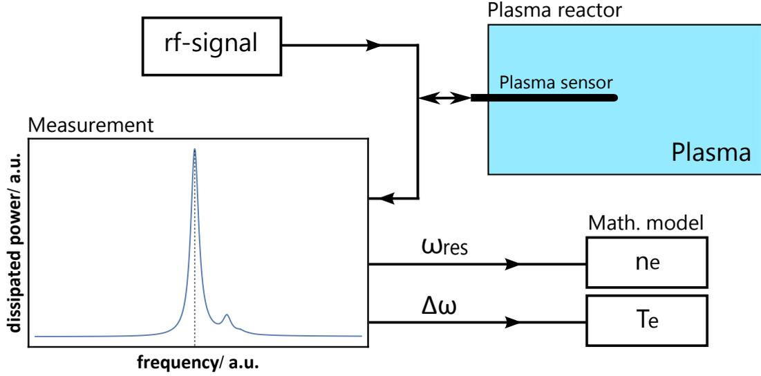
Figure 1.2: Schematical depiction of APRS: a radio-frequency signal is coupled into plasma via a probe, and the spectral response is recorded and analyzed. From the resonance curves, the corresponding plasma parameters can be determined by using a mathematical model.
