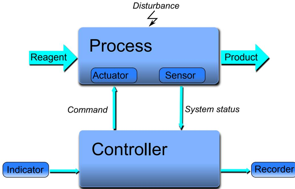
*Figure 1.1:* Control loop with disturbance of the process: The controller monitors the controlled process via a sensor. Depending on the captured system status, the adjustment can be executed by the actuator. The indicator sets the goal of the process, whereas the recorder collects the data.
