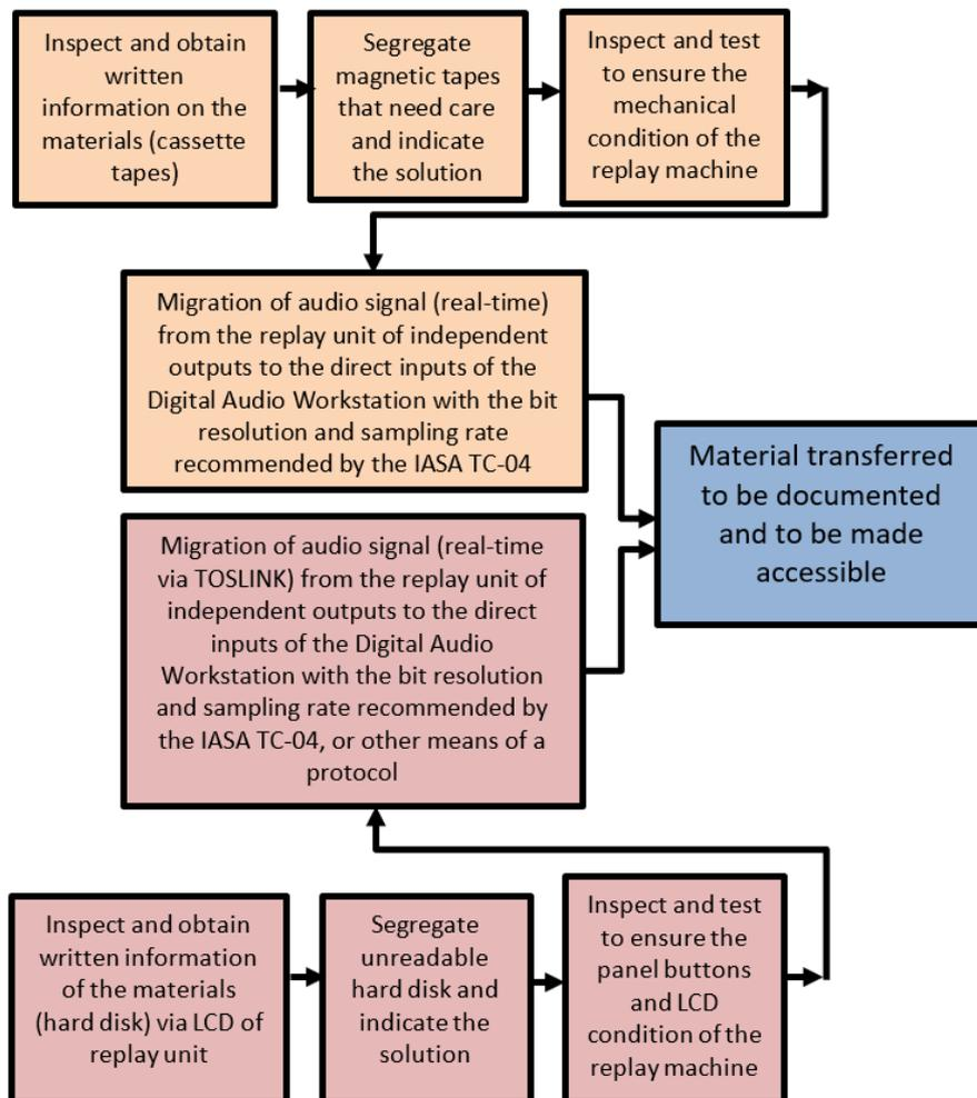
**FIGURE 6: Signal extractions of two different platforms, namely the multi-track cassettes magnetic tape and the hard disk recorder replay machine (scheme and all following schemes by the author).**
