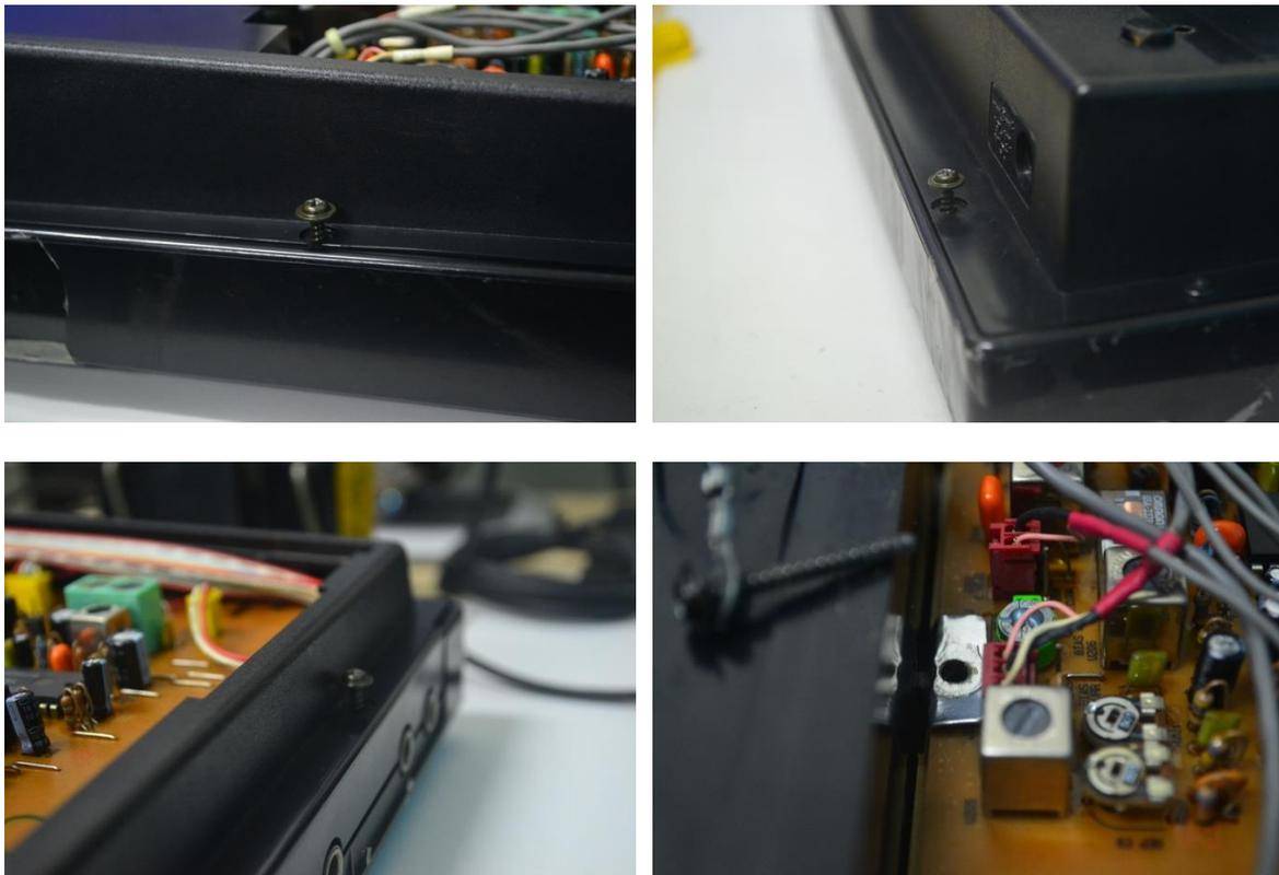
**FIGURE 13a, b, c, and d: Four screws have to be removed, with the last being attached to grounding of the circuit board.**
